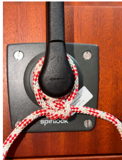
Figure 4 Wraps secured with a reef knot
